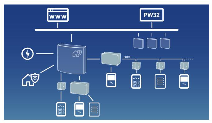
smartONE is an innovative security system where all data transmission occurs securely through encrypted and monitored two-way communication. In its basic configuration, smartONE does not require a connection to a server or separate software installation. The central unit has a built-in web server.
