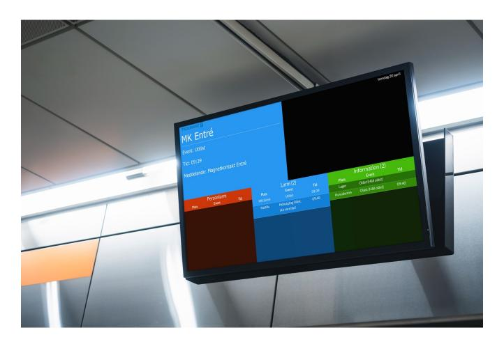
When no alarms are being presented on the alarm monitor, it can be used to display digital content. This can include a website, company logo, information board, or simply a beautiful image. When an alarm is activated, the monitor returns to alarm presentation mode.
